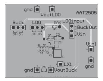
Figure 4: AAT2505 Evaluation Board Bottom Side.
