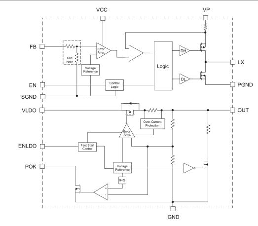
Note: Internal resistor divider included for 🗆 1.2V versions. For low voltage versions, the feedback pin is tied directly to the error amplifier input.
