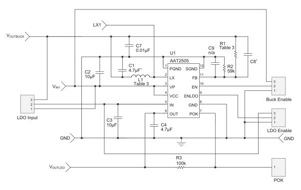
Figure 5: AAT2505 Evaluation Board Schematic.
