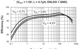
Step-Down Converter Efficiency vs. Load
