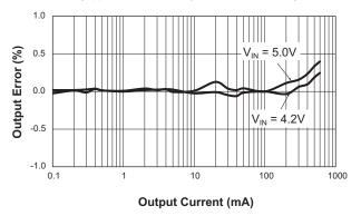
**Step-Down Converter DC Regulation**  $(V_{OUT} = 2.5V; L = 6.8\mu$ H; ENLDO = GND) 1.0 V<sub>IN</sub> = 5.0V Output Error (%) 0.5 ΪΗ  $V_{IN} = 4.2V$ 0.0 V<sub>IN</sub> = 3.6V -0.5 ++++ V<sub>IN</sub> = 3.0V -1.0 0.1 10 100 1000 1 **Output Current (mA)**
