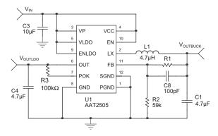
Figure 2: AAT2505 with Adjustable Step-Down Output and Enhanced Transient Response.
